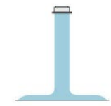
CEILING DIFFUSER IS POSSIBLE, NEED TO LOCATE WHERE PEOPLE ARE NOT FIXED IN PLACE TO AVOID DRAFTS
